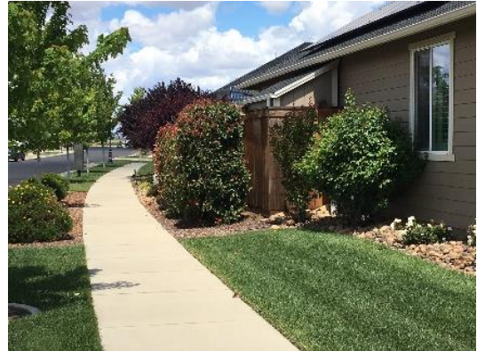
Five-foot side-yard fence setback from sidewalk to allow plantings to soften the fence and to not create a “wall effect” with a fence along the back of sidewalk.
